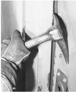
Work the **ADZ** into the stop between the door and jamb 6 inches above or below the lock push up or down causing the **ADZ** to rotate and create the door creating a **GAP**. The **PIKE** is used in conjunction with the adz to broaden its prying force against the door when gapping the door. It can also be driven into wood door jambs utilizing the baseball swing for forcing inward opening doors.
